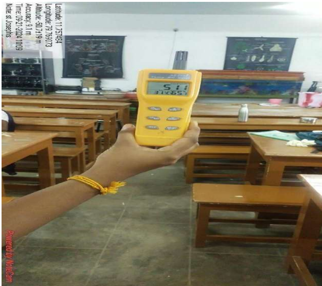
Carbon dioxide analyzer- Carbon dioxide level is low in the class room
