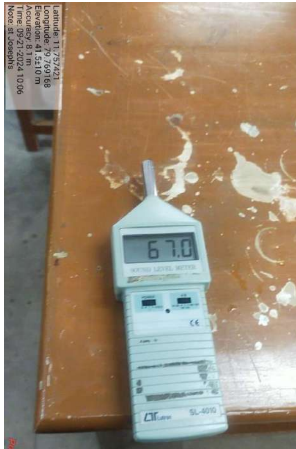
Sound Level Meter showing the Sound Level in the Classroom
