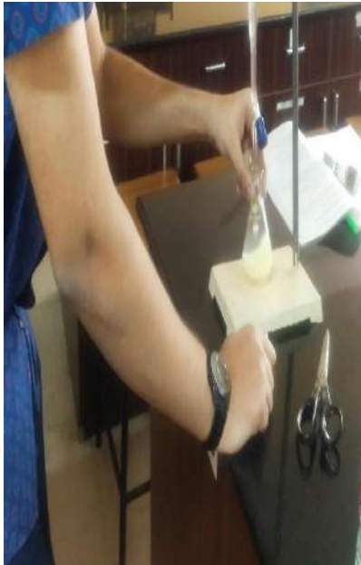
Chloride Analysis –Argentometric method
